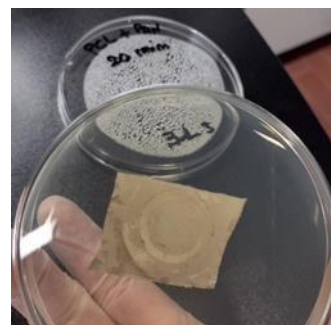
Figure 6 – Agar plate with PAN / PCL sample with 20 min deposition after 24h incubation
